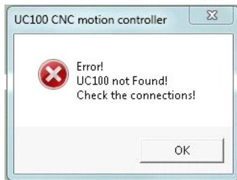
The following popup screen appears if Mach3 losing the connection with the UC100 meanwhile it is operating. This event may happen if the USB cable is broken or if the cable connector was accidentally slipping out from the UC100 or from the PC. The workaround is checking the USB cable connections and plug it back and restart Mach3.
