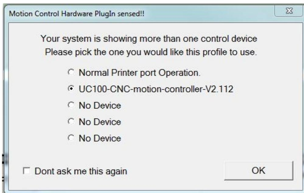
Select the UC100 CNC motion controller from the list.
